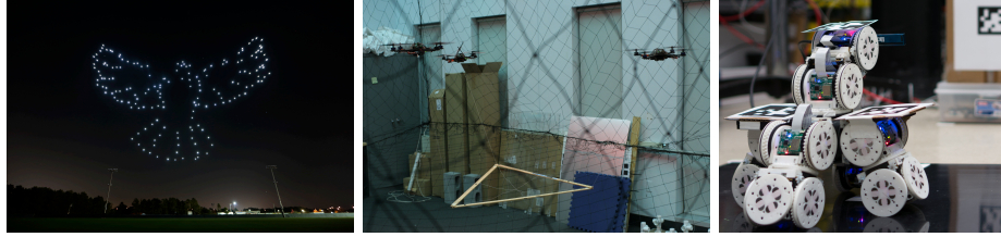
(a) 300 Intel Shooting Star drones performing choreography (Intel, 2017). (b) A team of quadrotors forming cooperative manipulation (Sreenath and Kumar, 2013). (c) The SMORES modular robot platform (Jing et al, 2016).
